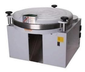
The BakeMax BMDBR01 Dough Ball Rounder can quickly round bread or pizza dough without strain. Portions ranging from 1.05 – 10.6 oz (30 – 300 grams) and comes with 3 interchangeable heads. The BMDBR01 is perfect for Bakeries and Pizza Shops.
